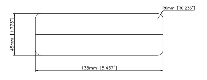
TOP AND BOTTOM DIMENSIONS ARE THE SAME EXCEPT FOR CASE ASSEMBLY BUSHINGS IN TOP (THREADED) AND THRU ASSEMBLY HOLES IN BOTTOM.
